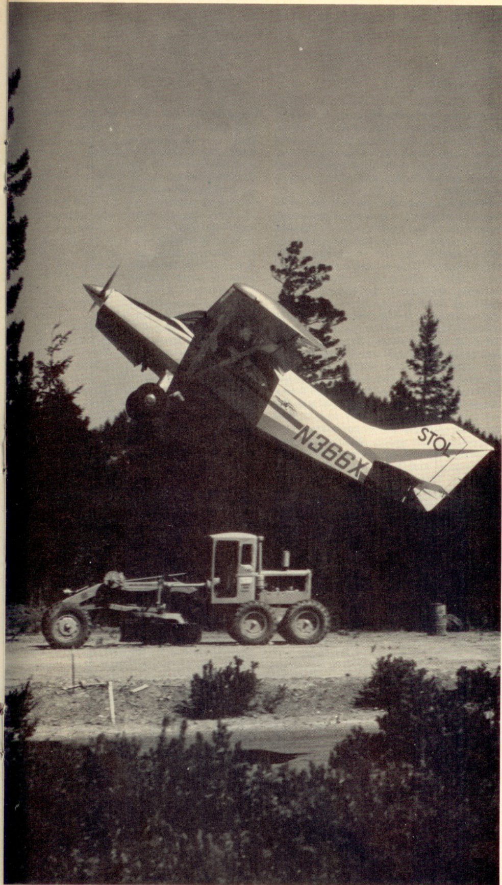
Maule in its element—a STOL liftoff from a bush-type airport. The new 235-hp Lycoming powerplant gets it off over 50 ft in 600 feet at 2,300-pound gross weight. Photos by author.
