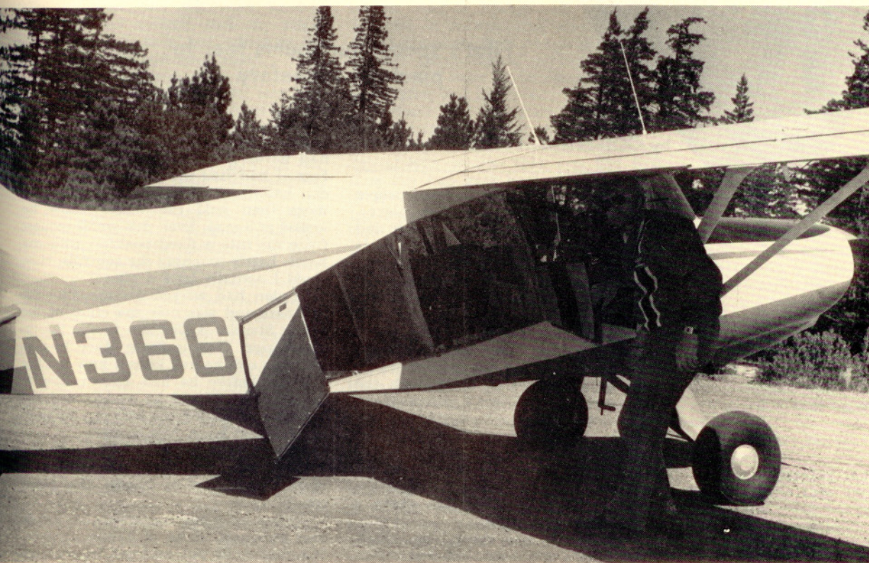
Maule distributor Joe Geiger opens ample, 51-inch-wide double cargo door. Rear seat can be folded or removed to take advantage of 900-pound useful load for freight. Extra large tires are for soft/rough fields.
