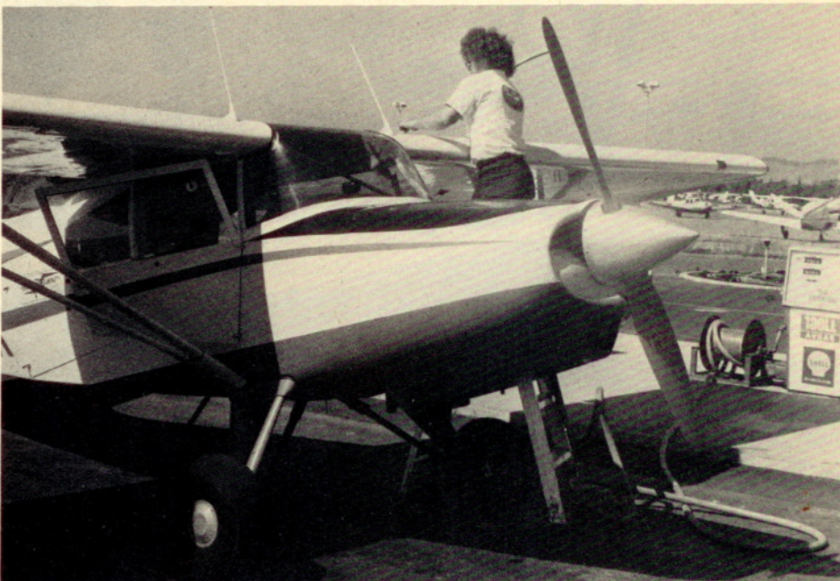
Conventional-looking high-wing "taildragger" Maule M-5 carries 43 gallons of fuel standard or 67 with aux tanks which boost range up to 990 miles at 65% power.
